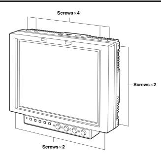
A total of eight cosmetic screws are provided with the monitor for use at such times when the main controls have been relocated. (Refer to page 9)
